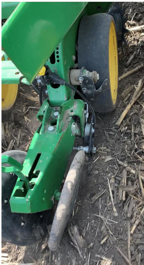
Photos 2 & 3. The 360 Bandit system installed on the 6-row research planter. The dribble treatment visible on the soil surface after planting.
