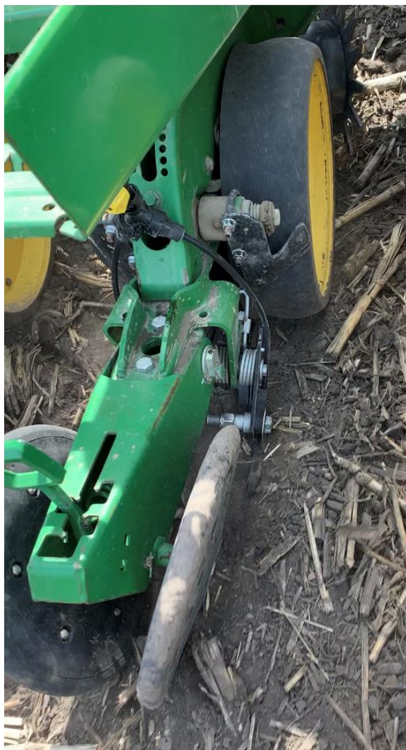
Photos 1 & 2. The 360 Bandit system installed on the 6-row research planter. The dribble treatment visible on the soil surface after planting.
