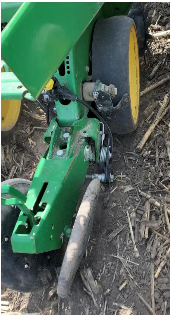
Photos 2 & 3. The 360 Bandit system installed on the 6-row research planter. The dribble treatment visible in the soil surface after planting at the Renville South trial.
